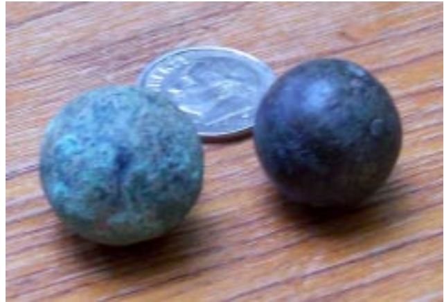
These two brass tumbling balls were found on the glen property by Jeff Vincent. They were used in the powder grinding process and possibly witnessed the last explosion. Their size can be compared to the nickel shown.
